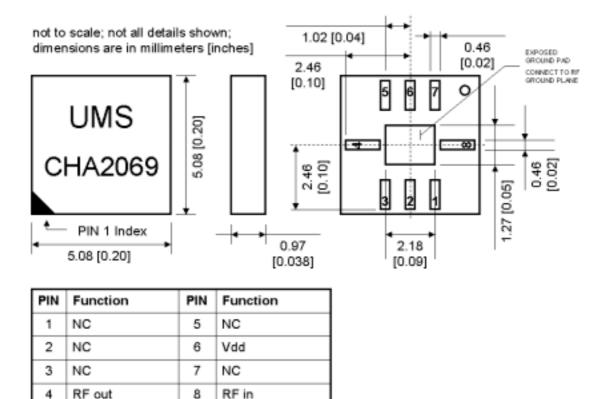
Please note that PIN 1 is located in the lower left corner of the package (front-side view) for all SMD-type packages from United Monolithic Semiconductors. It is indicated by a triangle on the package lid. Starting with PIN 1 the other pads are numbered counter-clockwise (front-side view). ATTENTION: The dot on the backside of the package (i.e. side with metallic pads) is just for fabrication purposes and does NOT indicate the location of PIN 1.
